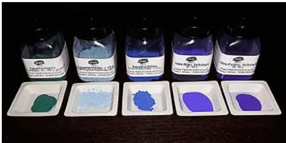
Fig. 8 Image of modern EB and related pigments marketed by Kremer Pigmente. From the left: 10,064 Egyptian green, 100,601 Egyptian blue (particles <math>< 10 \mu\text{m}</math>), 10,060 Egyptian blue (particles <math>< 120 \mu\text{m}</math>), 10,072 Han blue (i.e., CB) and 10,075 Han purple (i.e., CP) (colour figure online). Adapted from Nicola (2019)
