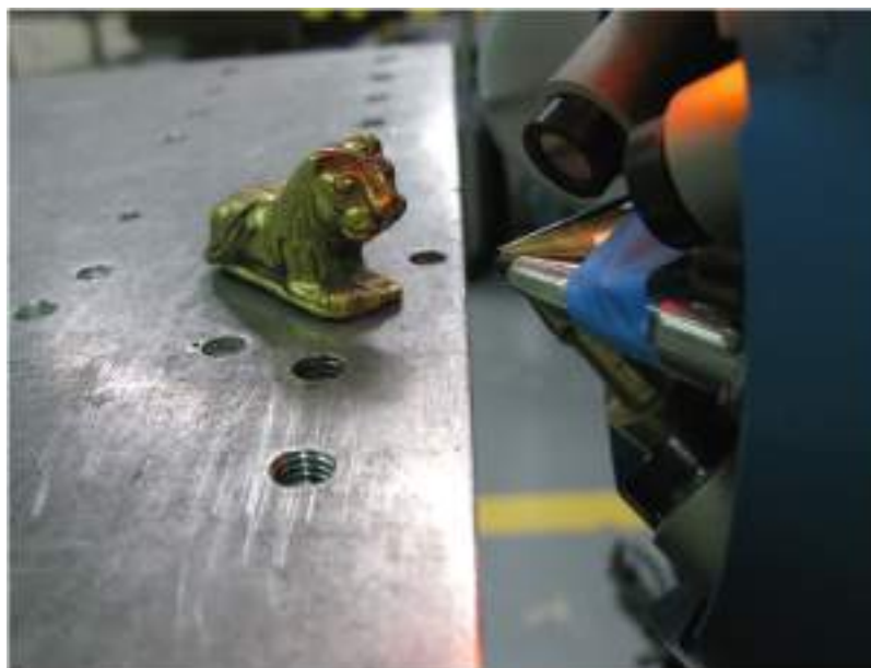
Fig. 2. One of the gold lions from King Ahmose's armband E7168 during \mu PIXE analysis at the extracted beam line of the AGLAE accelerator facility (C2RMF).
