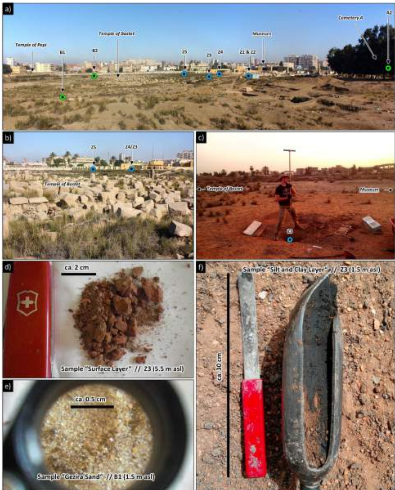
Fig. 3. Overview of drilling locations (2016 & 2018) and examples of sediment samples: a) panoramic overview of the excavation area and approximate location of the drilling locations, b) image of the Temple of Bastet, c) drilling in spring 2018 at borehole Z3, d) sediment sample “Surface Layer” taken at borehole Z3 in spring 2018 from a depth of 5.5 m asl, e) sediment sample “Gezira Sand” taken at borehole B1 in 2016 at 1.5 m asl seen through a magnifying glass, f) sediment sample “Silt and Clay Layer” taken in 2018 at borehole Z3 from a depth of 1.5 m asl. Images taken by T. Ullmann in 2015, 2016 & 2018.
