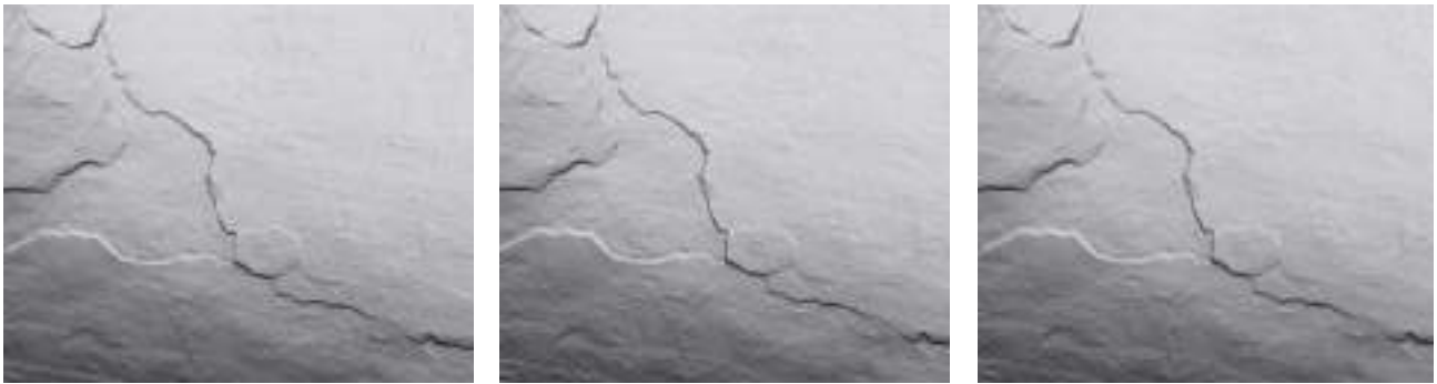
Figure 14. On the left, detail of the scanner model. In the centre, detail of the photogrammetric model from depth maps in high quality. On the right, detail of the photogrammetric model from depth maps in ultra-high quality.
