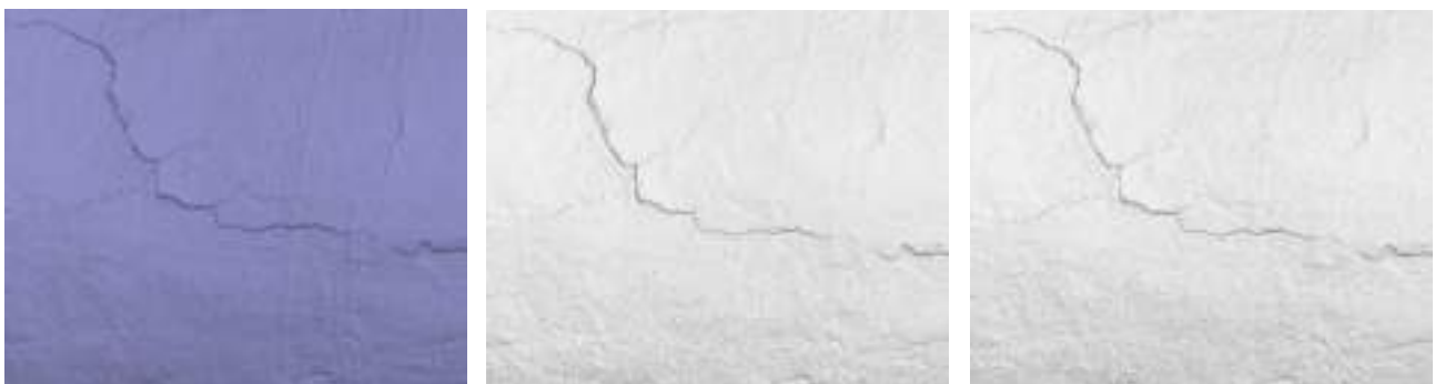
Figure 13. On the left, the mesh from the scanner survey. In the centre, The photogrammetric point cloud in high quality. On the right, the photogrammetric point cloud in ultra-high quality.
