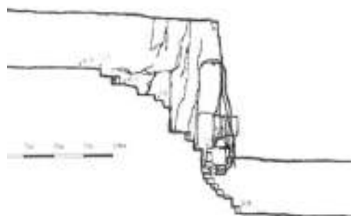
Fig. 7. Comparison section, showing the squared-off ceiling and (somewhat longer) staircase combination within another, earlier queen’s tomb: DB 320 (detail) (Graefe and Belova 2010, Plan 02 (edited detail), copyright © Nadejda Reshetnikova)
