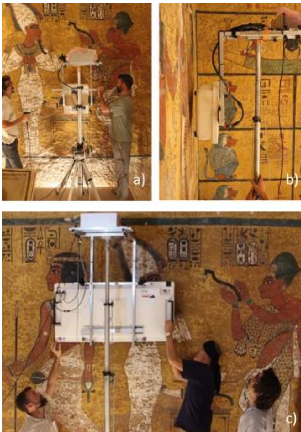
Fig. 3. Pictures taken during LF and IF radar scans showing: a) and b) the IDS TR200 shielded antenna and c) the multi-channel IDS Stream-C system deployed by the lifter.
