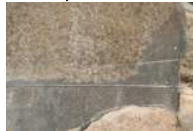
Fig.5 Cutting basalt by circular saw [12].
