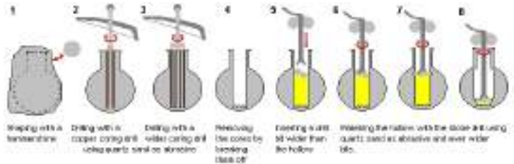
Fig.21 Procedure for producing a stone vessel [22].
