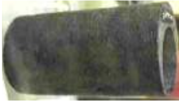
(b) Basalt tube cut by a tube drill.
