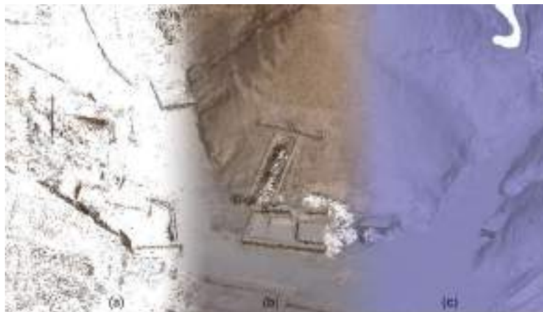
Figure 7. A picture presenting the different 3D photogrammetric products: Sparse point cloud (a) dense point cloud (b), triangulated mesh (c).
