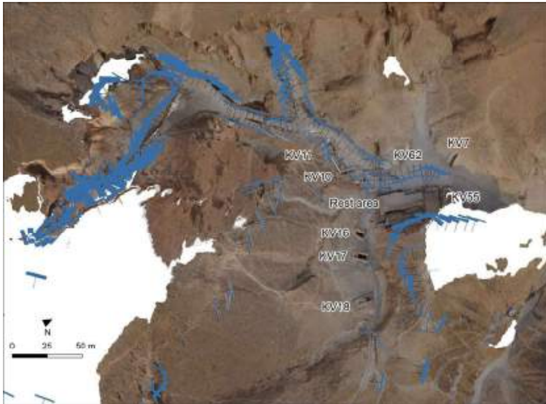
Figure 6. The position of the estimated camera centers after the photogrammetric block orientation, superimposed on the orthophoto generated from the subsequent photogrammetric process.
