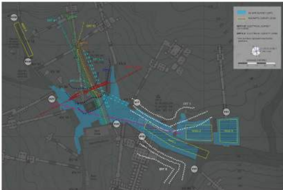
Figure 8. Map of the geophysical surveys performed in the area which contribute to the presented results. The different colored lines refer to the different Electrical Resistivity Tomography (ERT) surveys executed.
