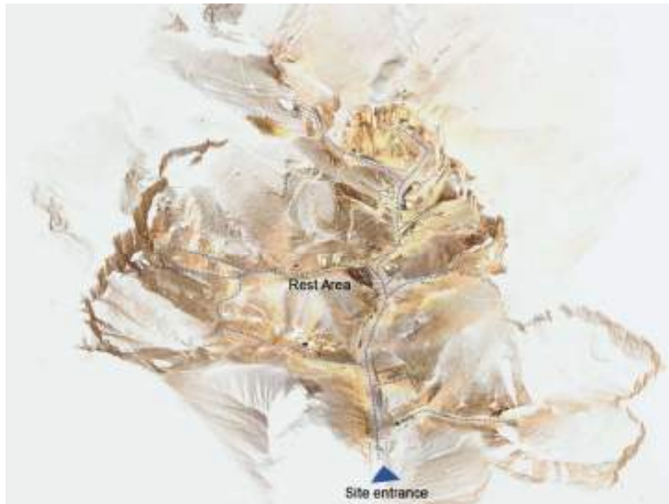
Figure 3. Image of the resulting merged point clouds (102 single scans) with more than 2 billion of points, and with superimposed visiting paths (open and closed).
